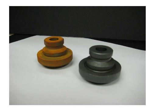
**Step 7:** 3:30 p.m. Cleaned part (at right) is dry and corrosion-free.
